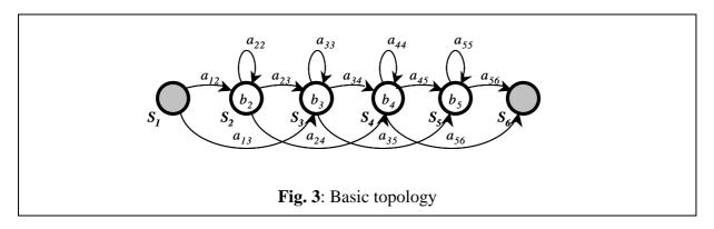
The models consist actually of 4 "active" states  $\{S_2, S_3, S_4, S_5\}$ : the first and last states (here  $S_1$  and  $S_6$ ), are "non emitting" states (no observation function), only used by HTK for some implementation facilities reasons. The observation functions  $b_i$  are single gaussian distributions with diagonal matrices. The transition probabilities are quoted  $a_{ij}$ .
